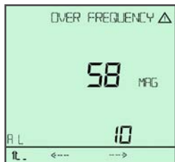
Alarm display showing active alarm*
