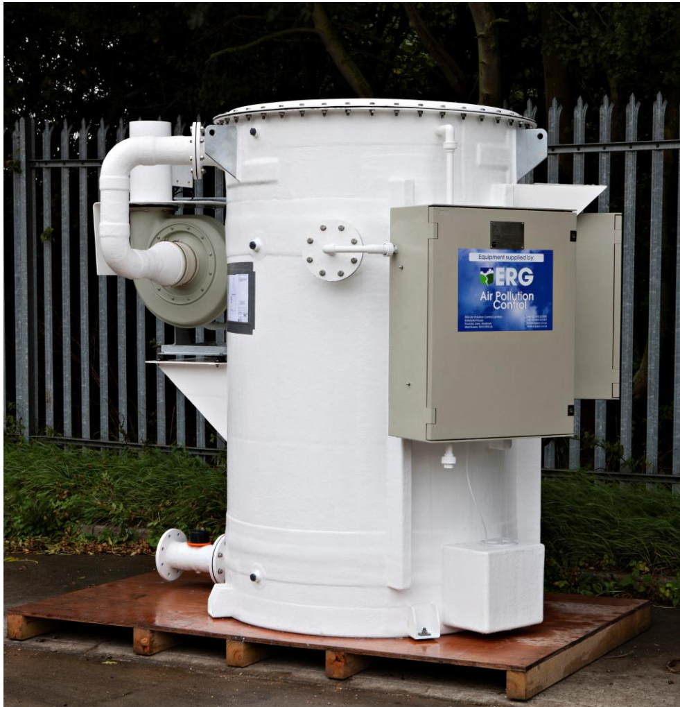
Modularised hybrid bio-scrubber / carbon filter unit destined for Iraq
