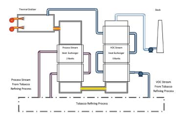
ERG Beverley were able to design and supply a thermal oxidiser – a vertical chamber – with a horizontal combustion chamber firing natural gas. The heat exchangers that were sourced from Beverley's partner company in the Czech Republic were of the tube bank design and incorporated significant thermal cycling design allowance.
