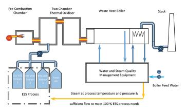
The system was specifically designed to allow periods of standby operation between shifts (6/24 h) without the need for cold starts and was able to tolerate intermittent emissions of particulate matter without causing long term damage to the plant.
