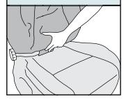
Fasten the side Velcro around the seat adjusters or armrests if applicable.
